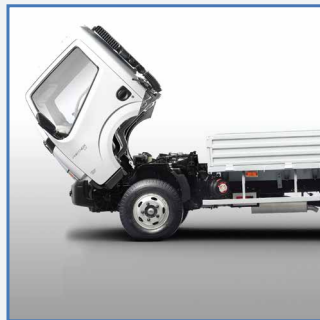
Tiltable cabin in any gear - ease of serviceability
