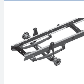
Front parabolic suspension with shock absorbers
