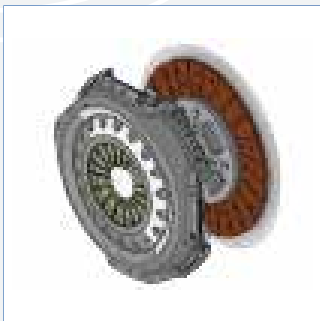
310 mm clutch with unilever type booster
