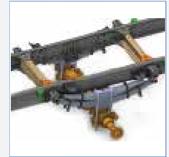
Rear heavy-duty semi-elliptical suspension with helper springs
